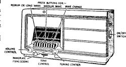
This cabinet houses the Mullard version. There are three buttons for wavechanging, three for medium wave pre-selected stations, . and three which can be set for either medium or long-wave programmes. The manual tuning knob is depressed for operation. A lever type of tone control is fitted.
